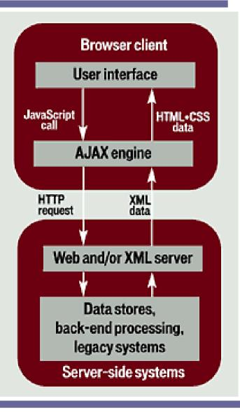
Communication between client and server is performed through an XMLHttpRequest
