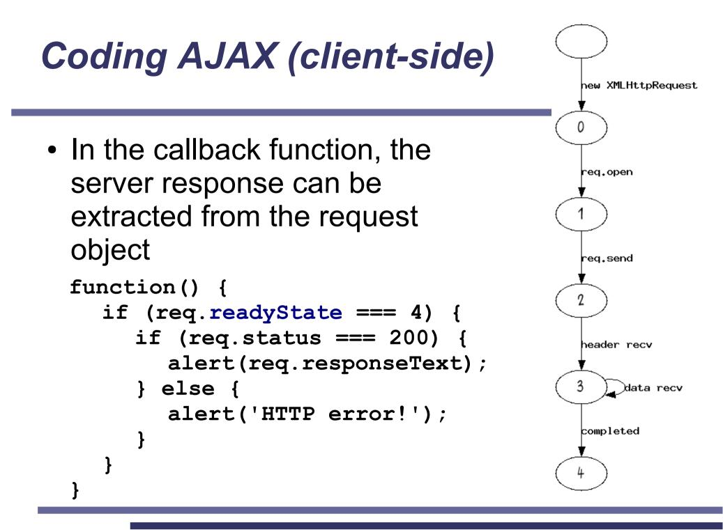
In the callback function, the server response can be extracted from the request object
